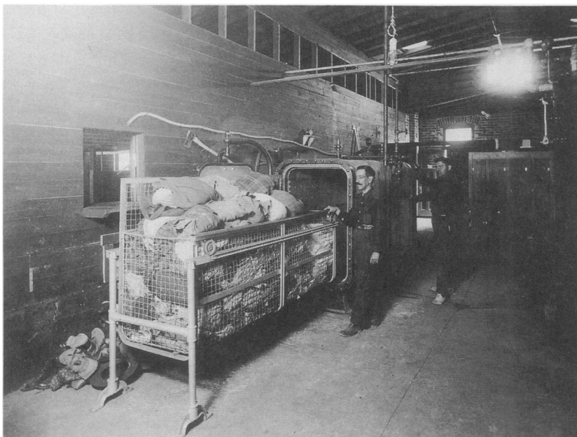
Photo 1: Steam disinfection of clothing at the Santa Fe Street Station. Photo included in letter from C. C. Pierce to Surgeon General, 16 Feb. 1917, NACP, USPHS, RG 90, CF 1897–1923, file 1248.
